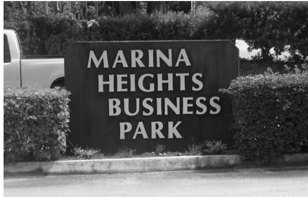
4 5 Figure 4. Example of a monument sign, one type of ground sign. 6
