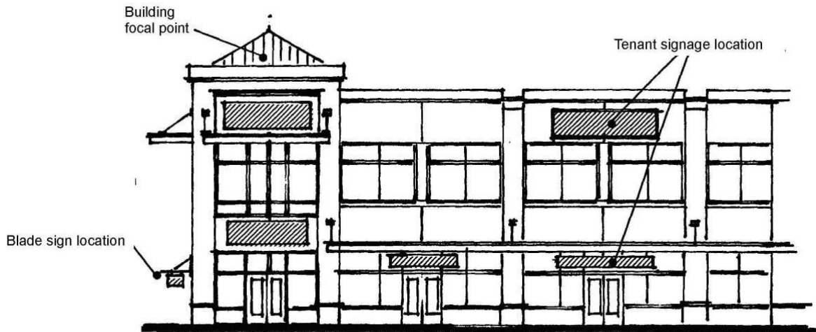
Figure 2. Appropriate sign location and size
